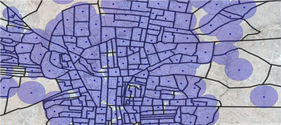
Figure C.2: Thiessen test polygons with bold boundaries representing the known enum. area boundaries.
